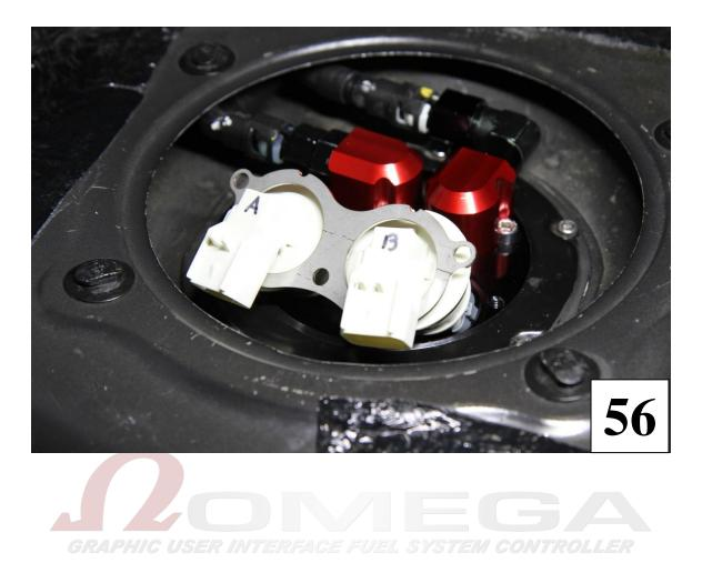
) Push the bulkheads into place on the top hat while aligning the pins. Make sure the O-rings are fully seated. Use the three cap screws and bolt the retaining plate into place.
