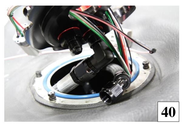
**41**) Install the return hose 45 degree -6AN fitting on to the top hat. Route the hose under the outlet fitting and hose of the filter housing. The fitting will be facing the right, passenger side of the tank when installed on the top hat. Make sure the hose does not point to the front in the tank. It may interfere with the level sensor. Pictures **# 45**, will show the inside tank hose and wire harness routing.
