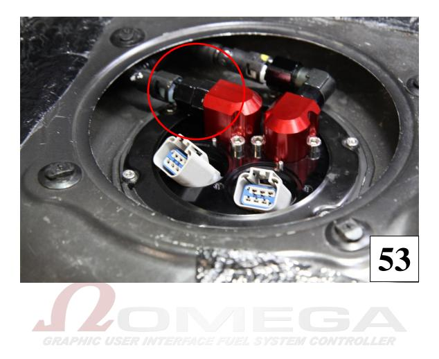
**54**) Locate the two electrical bulkheads. Make sure the O-rings are in the proper place. See the pictures for the location. Apply lube to the O-rings.
