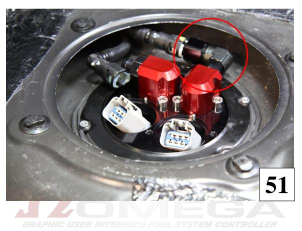
**51**) Install the female -8AN fitting onto the -8AN outlet port. Carefully tighten the fitting.
