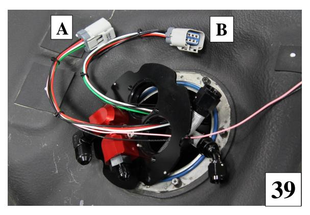
**40)** Install the feed hose straight -8AN fitting on to the top hat. It will need to be tightened so the fitting is pointing slightly to the right, passenger side. Level the top hat sending unit as it would sit on the tank to tighten the -8AN fitting. The straight fittings do not swivel so the orientation of where it is tighten is important to make sure the line does not twist when final installing the hat. Pictures **# 45** will show the inside tank hose and wire harness routing.
