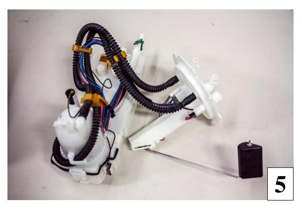
6) Once the sending unit is removed from the vehicle, removed the lower basket from the pump assembly. There are 7 clips that need to be released. Two small pocket screw drivers are usually best. You will also need to carefully remove the fuel temperature sensor.
