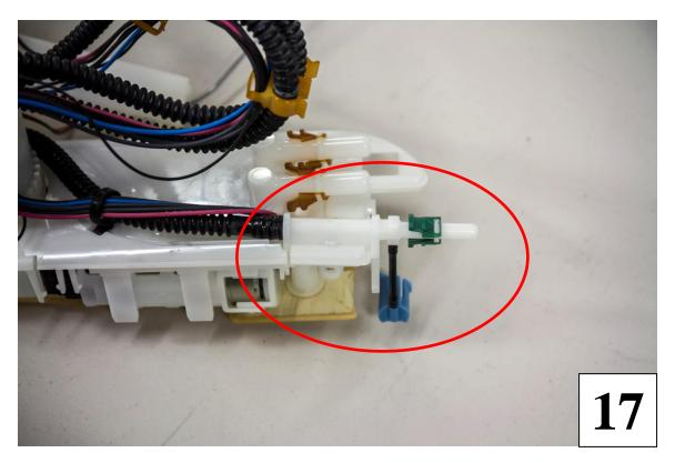
**18)** You will need to remove this part by carefully cutting the black hose off. Be mindful not to cut the barb as this part will be reused in the new Alpha brushless fuel pump system. Start by cutting off the black hose. A new sharp razor blade is best.
