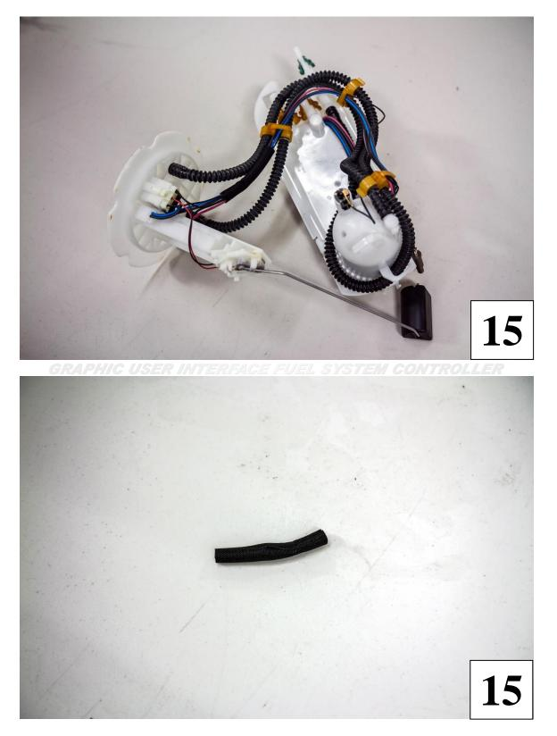
**16)** Apply the wrap to the new Alpha brushless pump harness and slide it down into the opening of the top plate. Use a supplied zip tie to secure the wrap in place. This will protect the harness from any chaffing.
