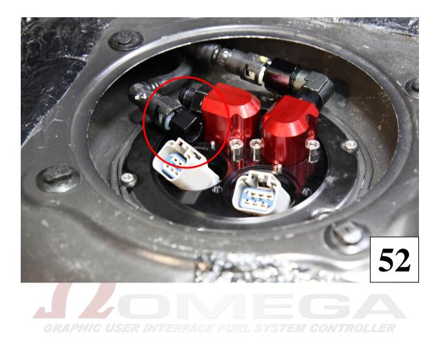
**53**) Install the female -6AN fitting onto the -6AN inlet port. Carefully tighten the fitting.
