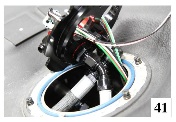
) Locate the fuel level sensor bracket and two M6 x 1.0 x 8mm cap strews. Slide the fuel level sensor into the bracket until it clips into place.
