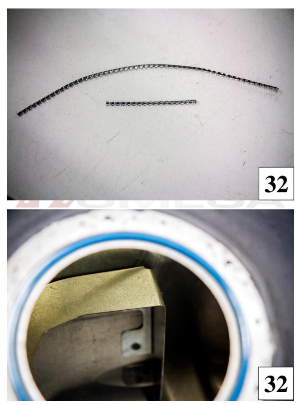
) Locate the 2 strips of Spring Fast metal edge protector. Install the protector on the edges inside the fuel tank as shown.
