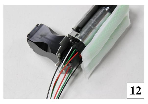
13) The Alpha brushless fuel pump assembly is designed to clip into the factory basket. Line up the tabs and make sure they fully clip into place.
