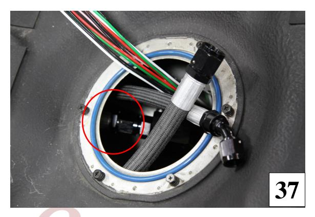
**38)** Locate the billet top hat. The Red bulkheads and fittings have already been installed for you. The electrical bulkheads are left out for now. They are the last piece to be install once the billet top hat is final installed.
