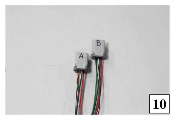
11) When assembling the fuel system, always keep **Connector A** on the **Right** side of the car and **Connector B** on the **Left** side of the car. This will aid in assembly, disassembly, and diagnosing if there ever is a problem.
