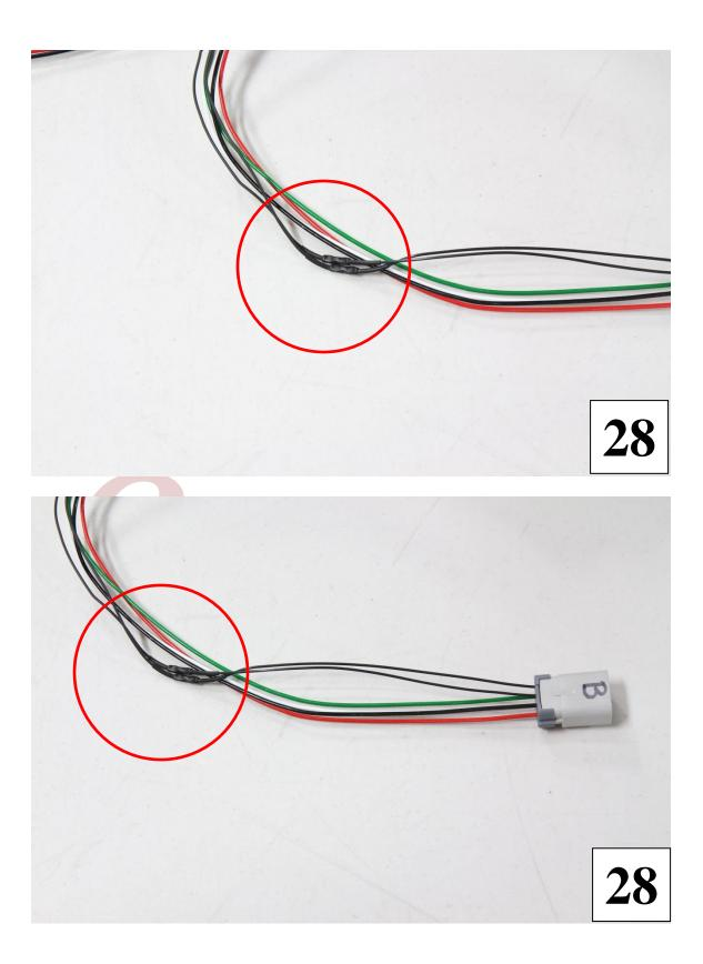
29) Next step is to wire the fuel level sensor to Connector A. Locate two 18-22ga barrel crimps and the 1/8" shrink wrap tubing. Cut two 1-1/2" pieces of 1/8" shrink wrap tubing. Leave the Pink and Black wires full length from Connector A and use the barrel crimps with shrink wrap tubing to make the connection at the fuel level sensor. Match the colors and connect the Pink to the Pink wire and the Black to the Black wire.
