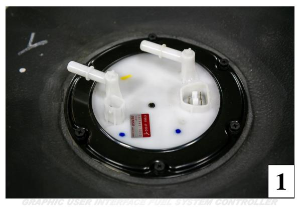
2) Make sure to drain all the fuel from the car before removing the sending unit. We offer a drain hose specific for GTRs to make draining simple and easy.
