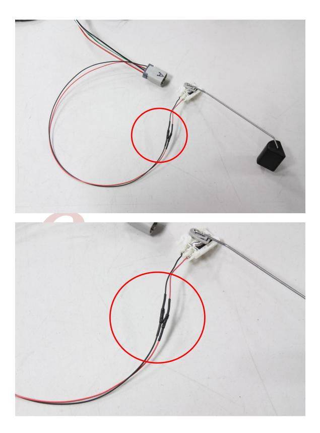
30) Use a couple zip ties to tie the fuel level sensor wiring together about half way to the 6 pin connectors. Place one zip tie approximately half way between the 6 pin connectors and the fuel sending unit assembly tying all the wires together on both harnesses. From that point, use zip ties to tie together the separate harnesses of Connector A and B. Do not tie everything together. Each connector will need about 12" of independence for installing the top hat in a later step.
