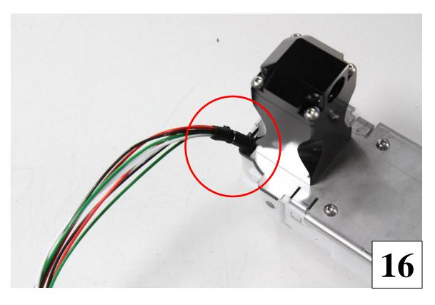
) Set the new Alpha brushless pump sending unit aside. Grab the factory fuel pump assembly and remove the syphon system pressure regulator from the assembly. It is the part with the smaller quick connect fitting.
