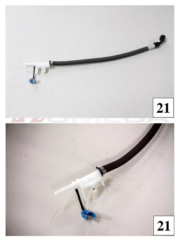
) On the bottom of the syphon regulator, there are 2 sets of clips. Remove the rear clips in the pictures shown by using a sharp razor blade or sharp side cutters.
