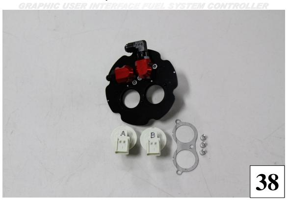
39) The next steps are to install the billet top hat. Start by slipping the inside tank harnesses A and B through the open ports. Connector A gets installed in the right side open port or Passenger side. Connector B gets install in the left side open port or Driver's side. The fuel level sensor is left outside the tank for now.
