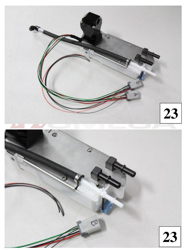
) Clip the syphon regulator and hose into place on the factory basket with the Alpha brushless fuel pump assembly.
