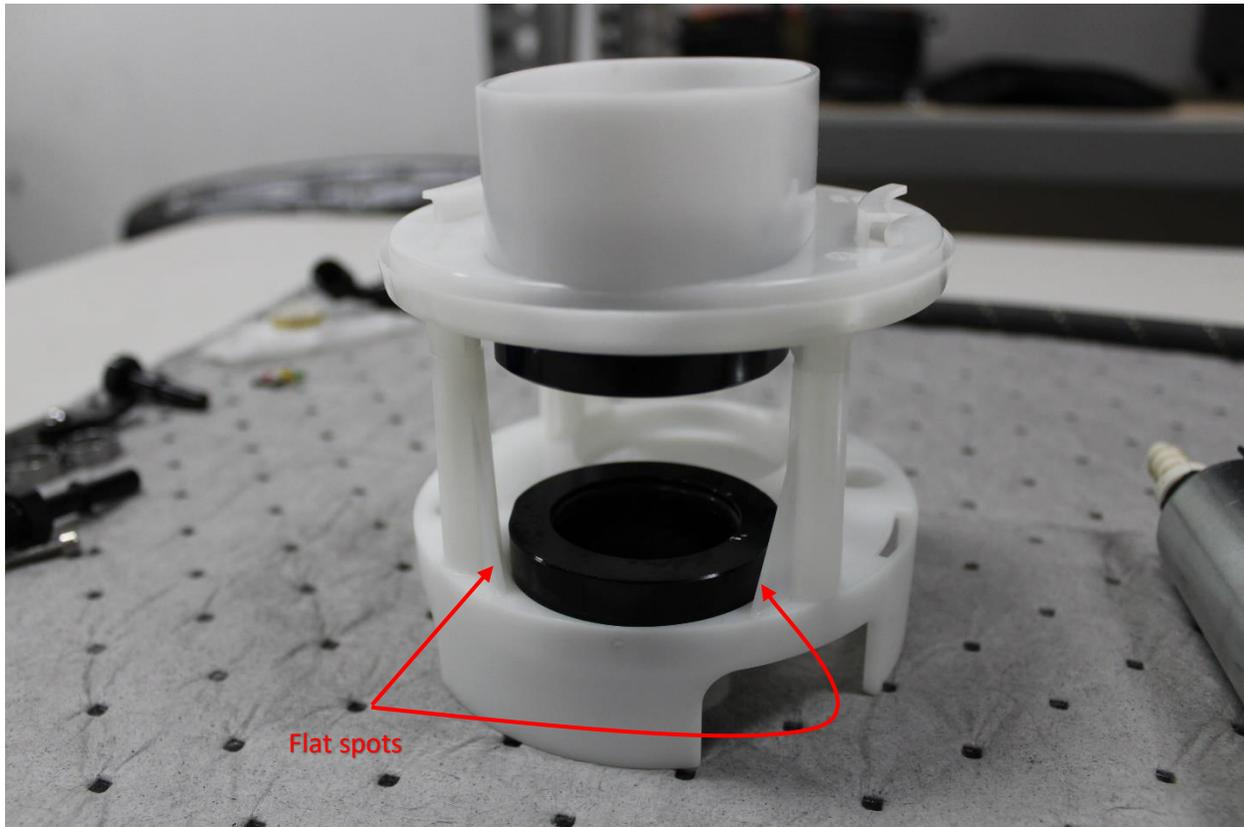
27. Lubricate the O-rings with a silicone spray or similar. Place the pumps into the basket until they sit all the way down while keeping the upper cap in position. Check that the machined flats are also in correct position. See photos for correct clocking of the pump outlet barb.
