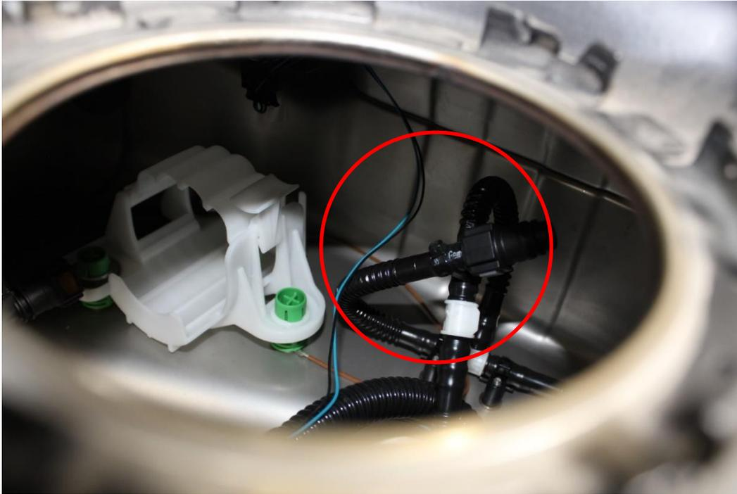
39. Gather the red top hat and fittings shown below. Lubricate the O-rings on the three fittings. Also, apply red loctite to the threads of the AN fitting and install them in the locations shown below.
