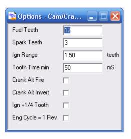
Make the following changes if you're running a 2-channel ignition in a wasted spark configuration:
